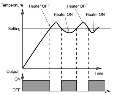
Two-position control (ON-OFF control) can be used to perform simple temperature control.
