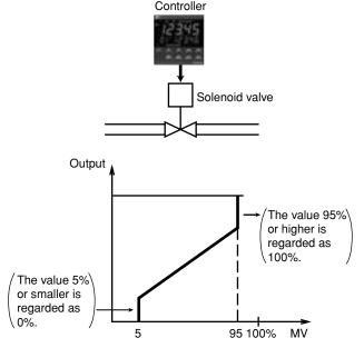
When solenoid valves are used, setting may be necessary to disable reaction when the MV value becomes less than a certain level. Use MV limit MH and ML (scale off) in such cases.
