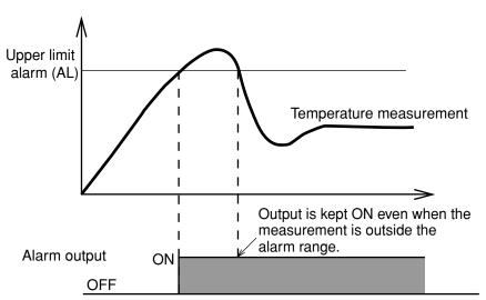
Once temperature measurement departs from the alarm range, the alarm output is set to OFF. To prevent this from occurring, the alarm latch function holds the output to ON even when the measurement does not fall within the alarm range. After checking the alarm, the operator can reset the alarm latch using one of the following methods:
