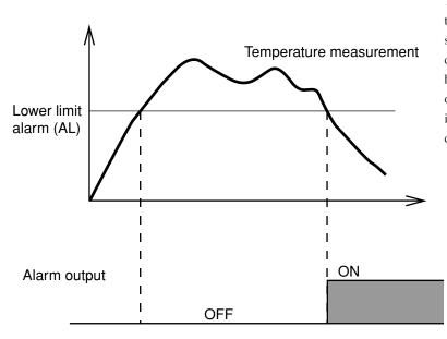
The temperature may fall within the alarm range from the beginning, such as when temperature control is started. In such cases, an alarm is issued at first under normal alarm operations. To avoid this, "with hold" can be selected. Then, after the power is turned on or the control is started, whether the temperature is outside the alarm range is checked, and then alarm detection is started.
