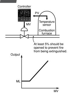
In some cases such as incineration control, MV should not be decreased to less than a certain level. Use ML (limit) of MV limit in such cases to prevent MV from decreasing to less than ML.
