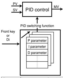
When manufacturing various products with only one machine, optimum PID parameters may vary depending on the products to be manufactured. In such cases, use the PID switching function. This function allows you to use sets of PID parameters specified beforehand, which can then be switched using the keys on the front panel or using Di.
