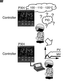
More accurate results can be obtained more quickly if PID tuning is performed while PV trend is checked.
