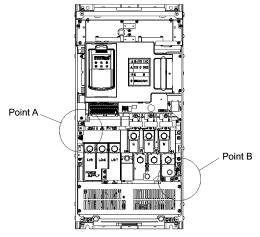
Figure 10.4 Internal Location Diagram (FRN110F1S-4J)
