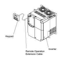
Figure 2.31 Installing it at a Remote Site (e.g. for Operation on Hand)
