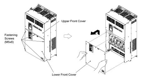
The lower front cover should be removed for wiring.
