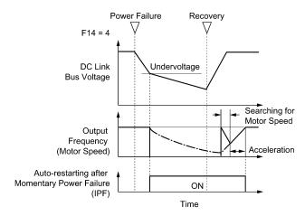
Restart mode after momentary power failure (Allowable momentary power failure time) (H16)
