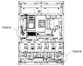
Figure 10.7 Internal Location Diagram (FRN132F1S-4J, FRN160F1S-4J)
