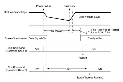
If you set the allowable momentary power failure time (H16) to "999," restart will take place until the DC link bus voltage drops down to the allowable voltage for restart after a momentary power failure as shown below. If the DC link bus voltage drops below the allowable voltage for restart after momentary power failure, the inverter recognizes that the power has been shut down so that it does not restart but starts (normal starting).
