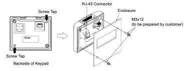
Figure 2.34 Mounting a Keypad on the Enclosure Wall
