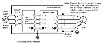
Figure 10.3 Installation of EMC-Compliant Filter (Option)
