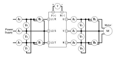
Figure 7.1 Connection of Meters
