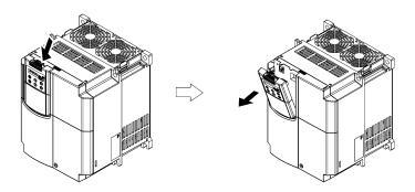
Figure 2.32 Removing a Keypad
