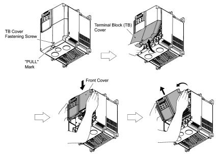
Figure 2.6 Removing the Covers (FRN15F1S-2J)
