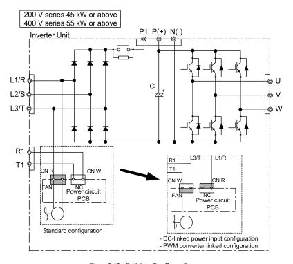
Figure 2.13 Switching Fan Power Source
