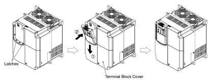
Figure 2.36 Retracting the Keypad
