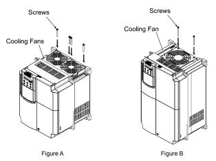
Figure 2.4 Fixing the Cooling Fan(s)
