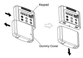
Figure 2.33 Separation of the Dummy Cover
