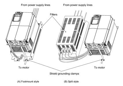
Figure 10.2 Installing Inverter and EMC-compliant Filter
