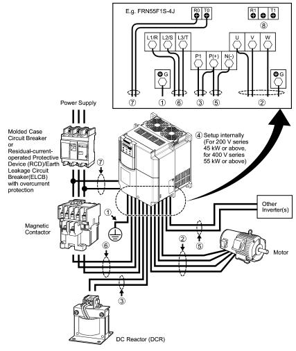
Figure 2.12 Wiring Procedure for Peripheral Equipment
