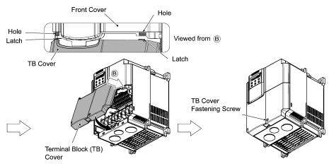
Figure 2.7 Mounting the Covers (FRN15F1S-2J)
