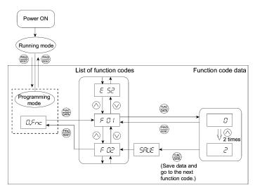
Figure 3.5 Example of Function Code Data Changing Procedure
