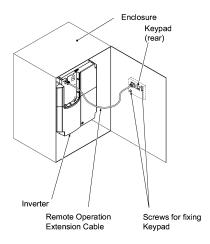
Figure 2.30 Mounting it on the Enclosure Wall
