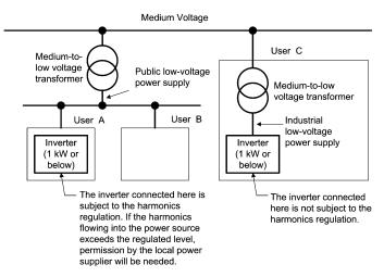
Figure 10.1 Connection to Power Line
