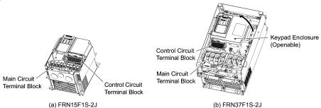
Control Circuit Keypad Enclosure Terminal Block (Openable) Main Circuit Terminal Block
