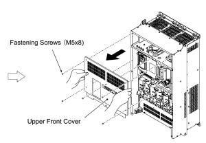
The upper front cover can also be removed as shown above.
