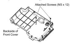
Tightening torque: 0.7 N·m
