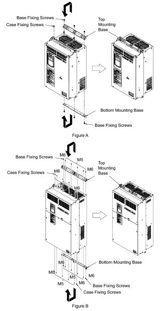
Figure 2.3 Relocating the Top and Bottom Mounting Bases
