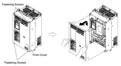
Figure 2.8 Removing the Front Cover (FRN37F1S-2J)
