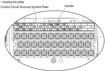
Figure 2.28 Closing the Control Circuit Terminal Symbol Plate
