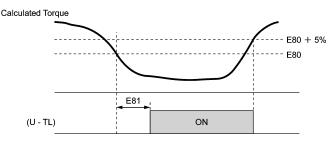
The detection level is set so that 100% corresponds to the rated torque of the motor.
