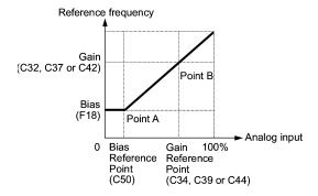
Example: Setting the bias, gain and its reference points when the reference frequency 0 to 100% follows the analog input of 1 to 5 VDC to terminal [12] (in frequency command 1).
