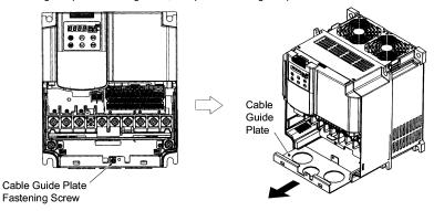
Figure 2.10 Removing the Cable Guide Plate (FRN15F1S-2J)
