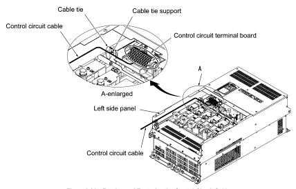
Figure 2.26 Routing and Fastening the Control Circuit Cable
