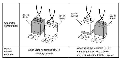
Figure 2.16 Reconfiguration of the (CN UX), (CN R) and (CN W) Connectors
